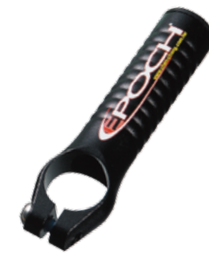
CC-EB28 Length 80mm Weight 60g Material AL6061T6 3D Forged Full CNC-machined Finish Anodized Color
