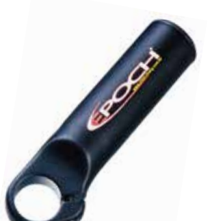
CC-EB33 Length 110mm Weight 155g Material AL6061T6 3D Forged Finish Sand Anodized Color
