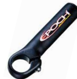
CC-EB31 Length 110mm Weight 115g Material AL6061T6 3D Forged Finish Sand Anodized Color
