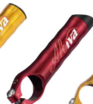
CC-EB24 Length 85mm Weight 52.5g/PR Material AL6061T6 3D Forged Full CNC-machined Finish Anodized Color
