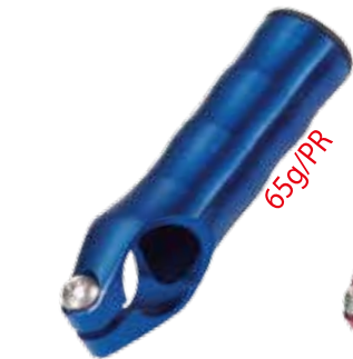
CC-EB25/25.4 Length 75mm Weight 65/55g PR Material AL6061T6 3D Forged Full CNC-machined Finish Anodized Color
