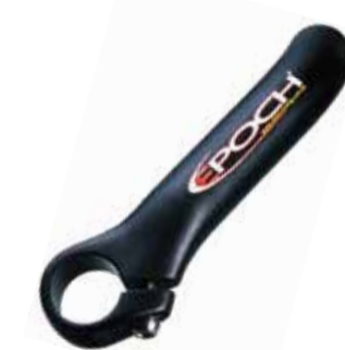
CC-EB30 Length 130mm Weight 140g Material AL6061T6 3D Forged Finish Sand Anodized Color
