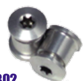
CC-CKB02 ■ Material AL7075T6 ■ Length M8-0.75X6.5L For Road M8-0.75X8.5L For MTB ■ Finish Anodized Color
