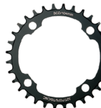
CC-FS32T 32T-38T Front Chainwheel Narrow wide tooth Alloy 7075T6 CNC Thickness 4.2MM For BCD 104mm
