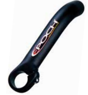
CC-EB29 Length 145mm Weight 135g Material AL6061T6 3D Forged Finish Sand Anodized Color
