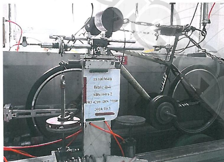
Fig. 5 Mechanical endurance test
